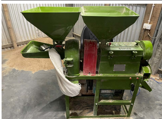
FIGURE 2 | Individual entrepreneur-run solar-powered rice mill with pulveriser combo machine in Nalbari district, Assam
