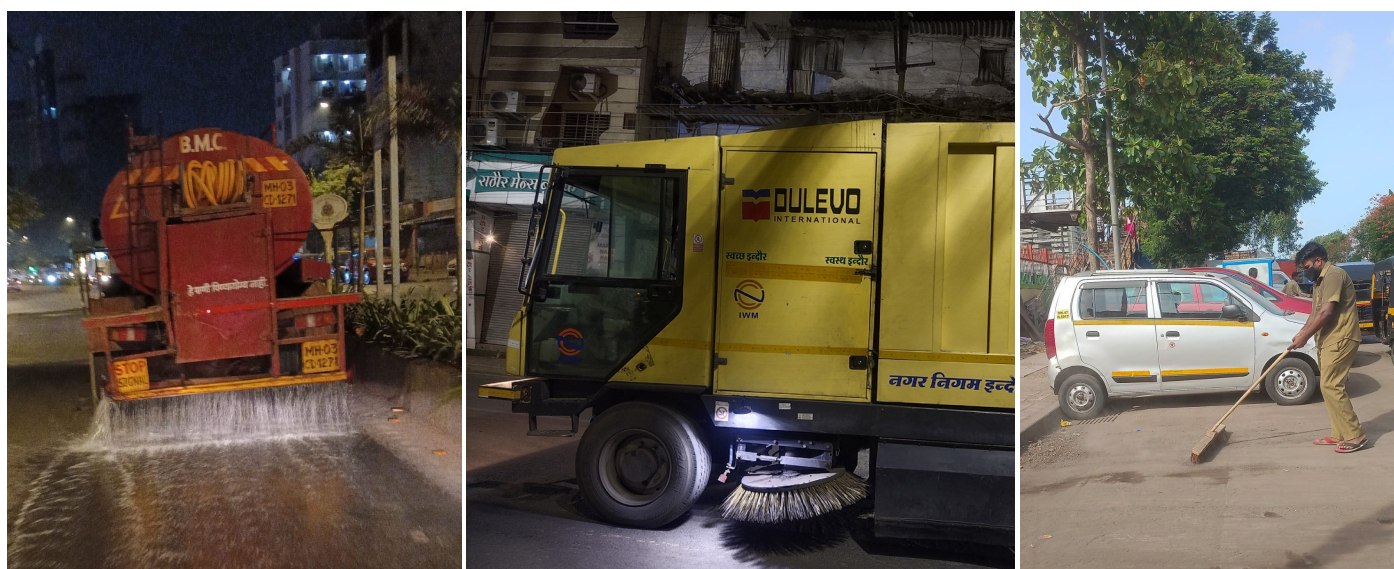
Figure 3 | Pictures showing water-based, mechanical, and manual cleaning of roads
