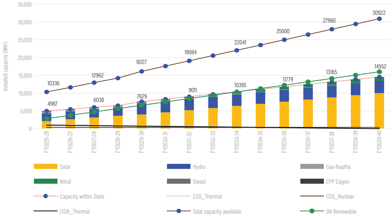
Figure 13 | Estimate of installed capacity growth: Zero Thermal 2040-Compensating (Balanced through RE Capacity Additions + OA RE) sub-scenario
